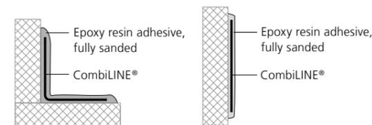
Simple and direct gluing of the expansion joint strip to walls and concrete foundations.
