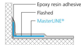
Horizontally flashed into the bituminous seal and vertically glued to the substrate with epoxy resin adhesive to form a force-fit, run-free connection.
